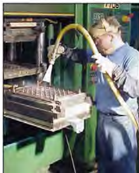
Cold Jet L.L.C. dry ice blasting technology is used to clean a production mold. Cold Jet says its products are both cost-effective and environmentally friendly.
