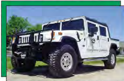
Hummers aren't known for fuel economy, but this one uses Gates Corp.'s H1 Hydraulic Hybrid Drive system, which replaces a vehicle's traditional motor system with a hydraulic pump that drives a hydraulic motor for propulsion. It offers a potential fuel savings of between 50 to 70 percent, the company said.
